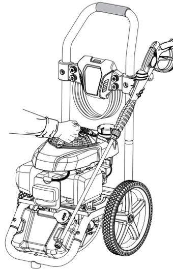
6 Allow engine to run for several seconds, then move choke to OFF (RUN) position (see page 10).
