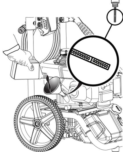
Turn the fuel valve to OFF before adding lubricant.
