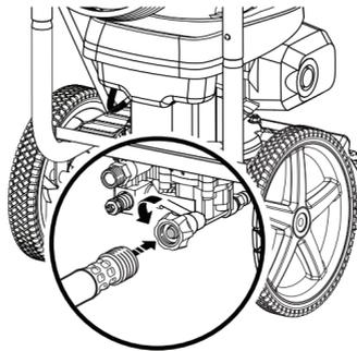
Completely uncoil garden hose or remove completely from reel to prevent kinks.
